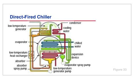
Next, the refrigerant travels through the condenser, expansion device, evaporator, and absorber in a manner similar to refrigerant travel in the indirect-fired double-effect absorption chiller.
